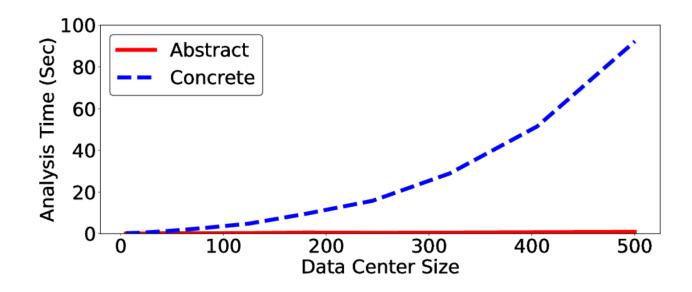
Simulation time vs. data center size for verifying all-pairs connectivity
